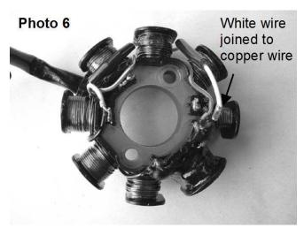
7. Slide the second sheathing strip over the crimp connection you just made. Route the new white wire so it follows the same molded guides as the red/white wire. Try to take as much loose slack out of the white wire as possible so it wraps tightly
