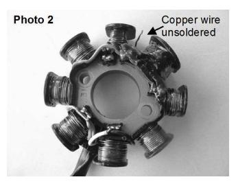
3. Locate the tab on the stator that the yellow wire attaches to. Unsolder the yellow wire from this tab. Do not unsolder the two copper wires attached to the same tab. Strip the end of the yellow wire so ½" of bare wire is showing. See Photo 3.
