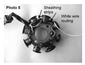
6. This step is the trickiest. You must cut the white wire to length, strip the end 1/4", and attach it to the freed copper wire using the remaining crimp connector. Hold up the white wire and cut it to length so that you have just enough slack to join the two wires. The goal is to leave as little slack in the white wire as possible once both are joined. See Photo 6.
