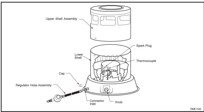
Fig. 1 Convection Heater parts identification.
