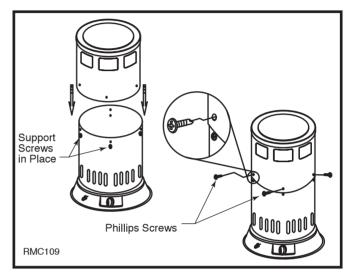
Fig. 4 Attach top with four phillips screws.
