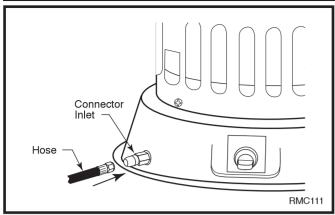
slowly. NOTE: If not opened slowly, excess-flow check valve on propane tank may stop gas flow. If this happens, you may hear a click inside the regulator assembly, this is the check valve closing. To reset the excess-flow check valve, close propane supply valve and open it again slowly.
