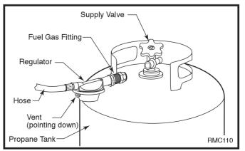
Fig. 5 Attach regulator with vent pointing down.
