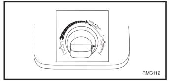
Fig. 7 Convection Heater control knob.
