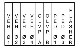
3.8.12.0 The flasher and load switch sockets shall be wired in the following arrangement in a twelve position back panel cabinet:
