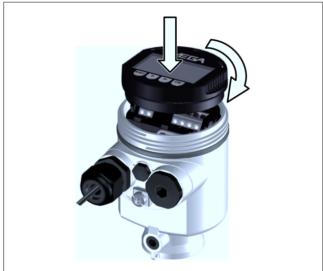
Fig. 21: Insertion of the indicating and adjustment module with single chamber housing into the electronics compartment
