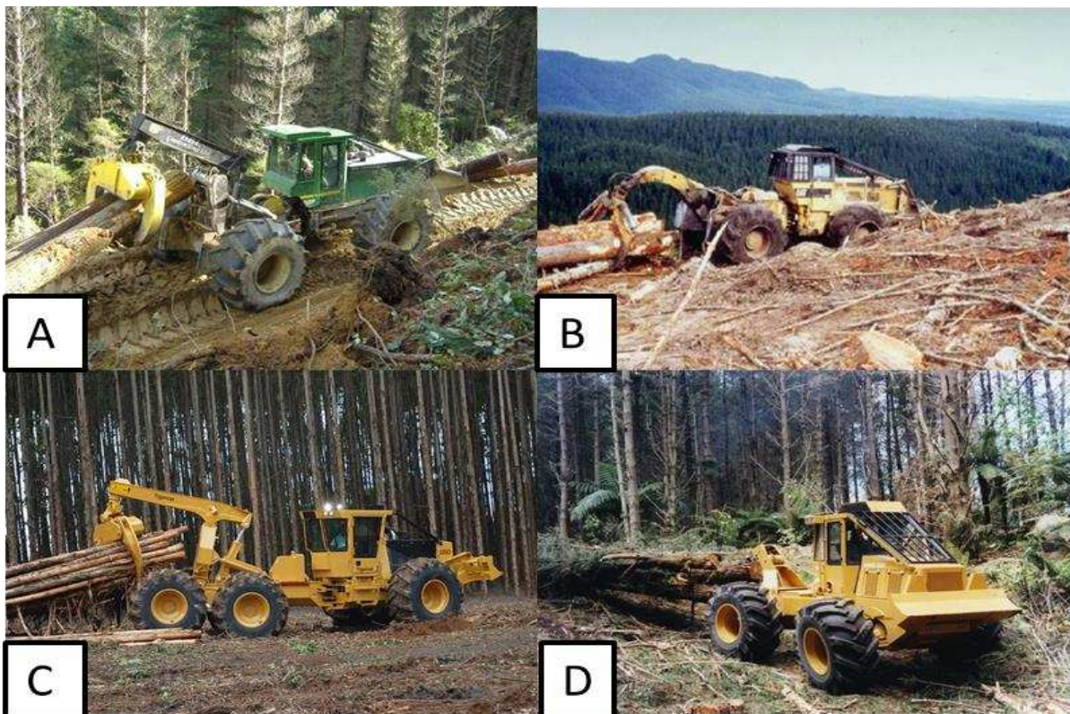
Figure 7: Skidding on different harvesting sites and surface moisture conditions. Skidders: A skidding uphill on moist conditions, B uphill on dry conditions, C on a flat site on wet site, and D downhill under dry surface conditions
