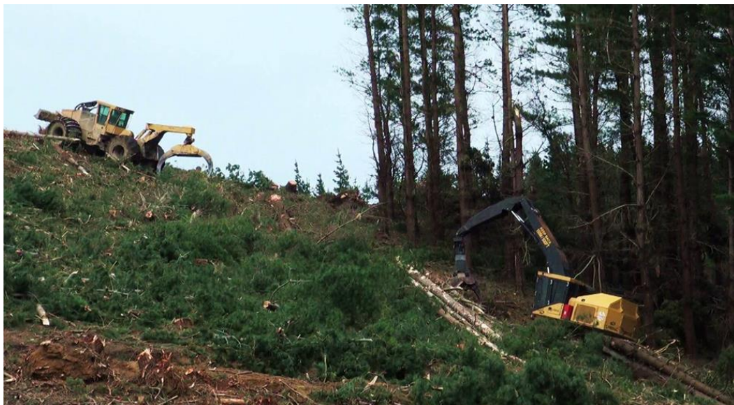
Figure 6: Skidder operation on a rolling site
