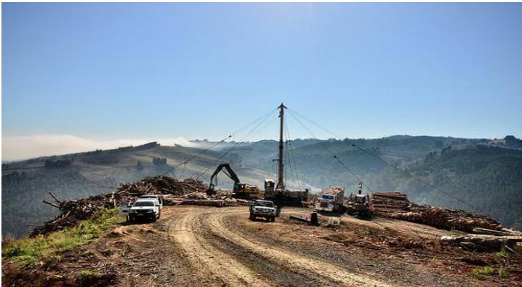
Figure 5: Typical CY set up in a steep country
