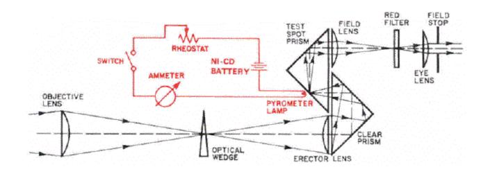
A typical optical pyrometer specification by PYRO
