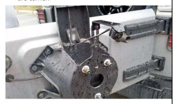
Adjustment Bracket for Camera Clearance using Phillips Screwdriver and 3/8" Wrench or Socket Drive
