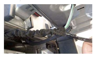
12. Finish running the harness to the front glove box area on the passenger side of the vehicle.
