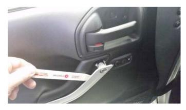
5. Remove the (2) Torx in the lower front of the door.
