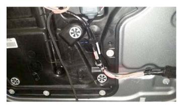
22. Run the camera wire through the factory door sleeve. Use a long zip tie or a fish tape.
