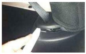
9. Using a plastic trim removal tool, remove rear access panel to expose 10mm bolt, and remove bolt.
