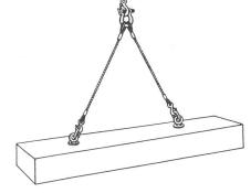
9. What is the minimum size of chain slings required to lift a load of 12,000 pounds? The two – leg bridle is in a choker hitch configuration at a 45 degree angle.
