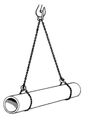
10. What is the minimum size of web slings required to lift a load of 8,000 pounds? The two slings are in a basket hitch configuration at a 60 degree angle.
