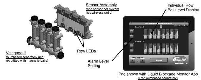
The premium system uses sensor assemblies mounted behind the Visagage flow monitors to sense where magnetic balls are floating in each row during liquid application. One of the sensor assemblies contains a wireless radio which communicates with the tablet (used as the control panel) in the cab. The tablet allows the user to select at which level on the Visagage the alarm will sound when a ball drops to or below that level.
