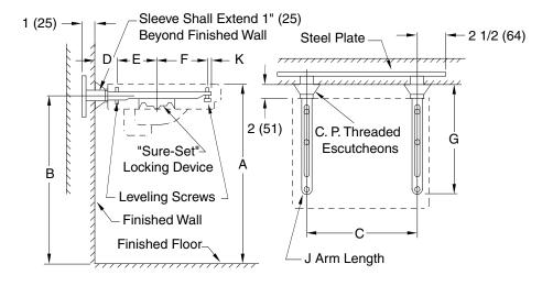
Fig. 0722 (-E) ... FOR FLAT SLAB LAVATORIES SET ON STEEL PLATE SECURED IN WALL
