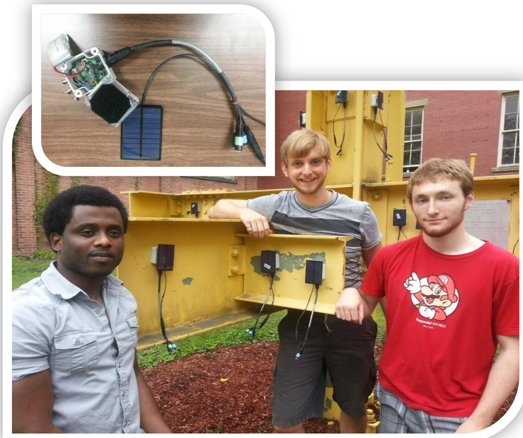
Wireless sensor nodes constructed by Project 3.3 researchers using a Zigbee development platform. (Left to right: students Gift Owahu, Ryan MacDonald and Erik Hatfield)
