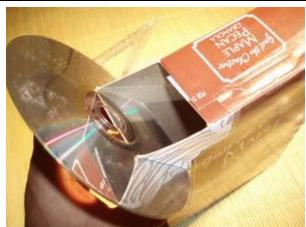
7.) Now you're going to cut a rectangle out on the opposite long side of the box as shown. The rectangle should be the width of the box and one inch high. The top of the rectangle should be about half an inch from the top of the box.
