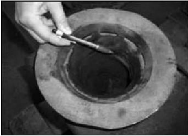
Fig. 10 Cleaning the burner knee off carbon deposits (only for pellets)
