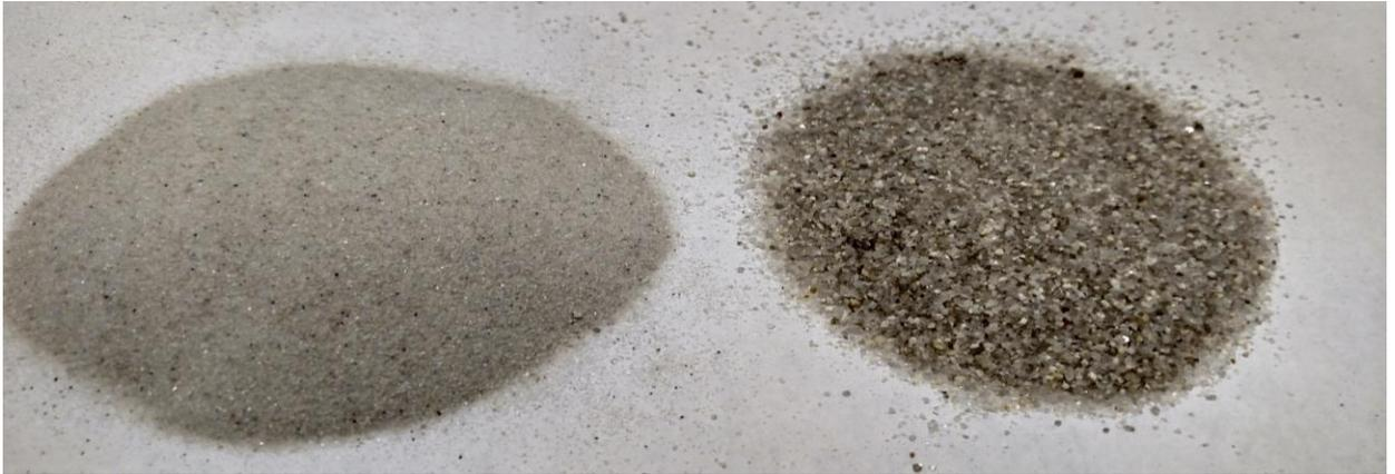
Figure 5.3 Photo of the two sand sizes tested. The fine grained sand (7030, left) and the coarser grained sand (4095, right) are pictured.
