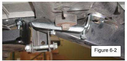
at the back of the bracket to hold it down while tightening the nut.
