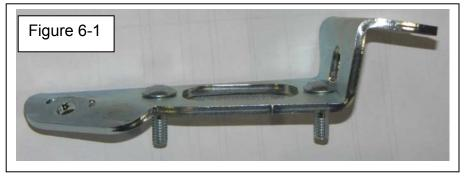
hammer to make a small dimple in this area to lessen the interference or take ~1/16" off the dome of the carriage bolt's head with a grinder/sander (not too much!) – but don't do either to the point where the bolt is loose – it should be 'trapped' between the bracket and frame when the bracket bolts are tight. For each side, reinstall the two
