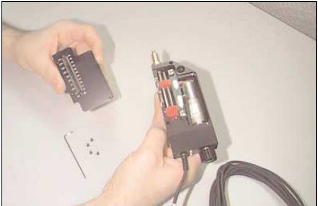
Figure 2: Approximate travel range markings assist in quick travel adjustment
