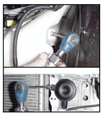
6. Remove three bolts that hold windshield washer tank and also remove bolt that holds horn and let horn hang. **NOTE:** The horn bolt will not be reused.
