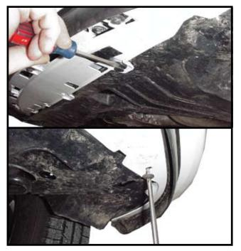
3. Remove eight plastic push fasteners from bottom side of facia and one screw from each side that attaches to wheel well extension.
