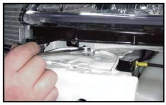
**5.** Remove six bolts that hold bumper on, four on the top side and two underneath. Set bumper aside temporarily.
