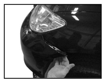
**4.** Pull facia straight out on each side by fender and carefully pull facia off.
