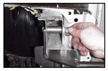
9. With an assistant, slide base plate on frame and install 1/2" x 3-1/2" bolt through base plate and previously installed spacer bushing. On inside of frame, use heavy frame washer with the flat side of the washer facing to the front of the (as shown on cover) car, 1/2" lock washer, and 1/2" hex nut. Do not tighten. NOTE: Use LOCTITE. Blue on all bolt threads.
