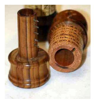
Trial fit the pieces again and check the operation and make any last adjustments before final assembly and finishing. Before installing the code rings carefully wax the backbone tube where the turning rings will be, leave the area for the fixed ring unwaxed for gluing. Finish the assembly and finish your Cryptex.
