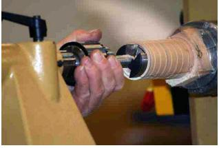
Next came the backbone tube, this is the piece that forms the structure for the turning rings. Again start by forming a tenon for mounting the tube in the chuck. Once mounted in the chuck bore it out
