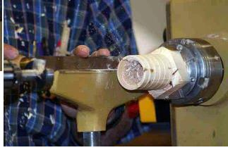
using a 1 1/8" Forstner bit, starting with out an extension initially then add the extension to finish getting the full depth needed. Now urn the tube down to 1 1/2" diameter using the cone center in the tail stock for support. Leave flats near the chuck to make drilling the pin holes easier.
