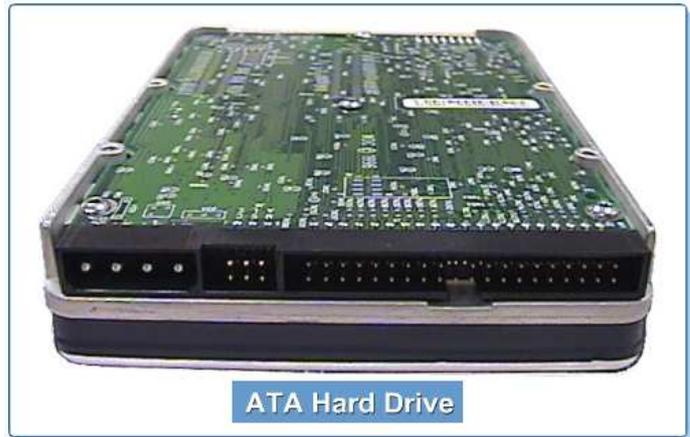
Upgrades to ATA disks generally fall into two categories. They are adding disk drives and replacing existing disk drives with faster or larger disk drives.
