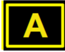
Taxiway Location Sign
