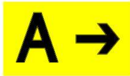
Direction/Runway Exit Sign
