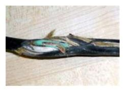
Inspect each tool carefully before you use it. If there are cracks, cuts or abrasions on the cord take the tool out of service until an electrician can replace the cord. Don't try to fix it yourself unless qualified to do so.
