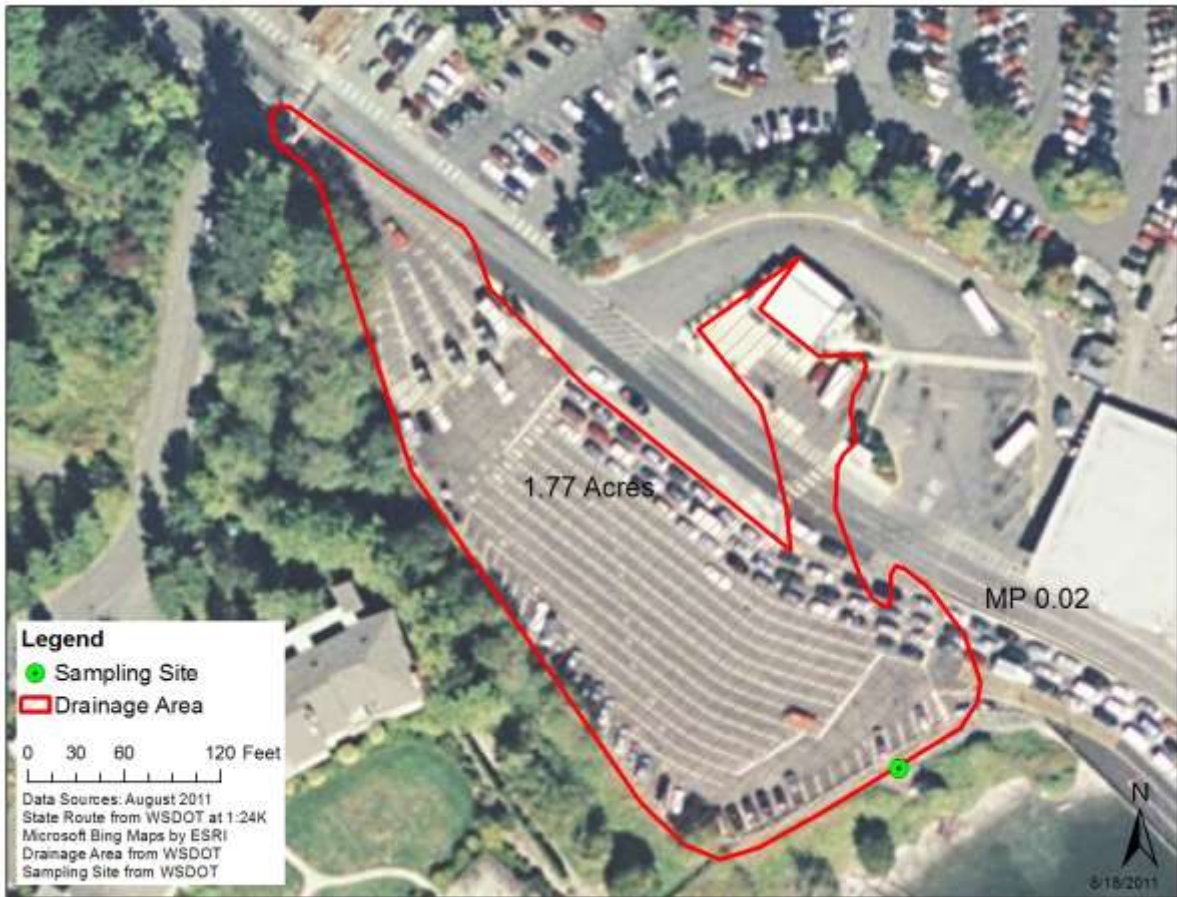
Figure D-9 Bainbridge Island Ferry Terminal sampling location and contributing drainage area.
