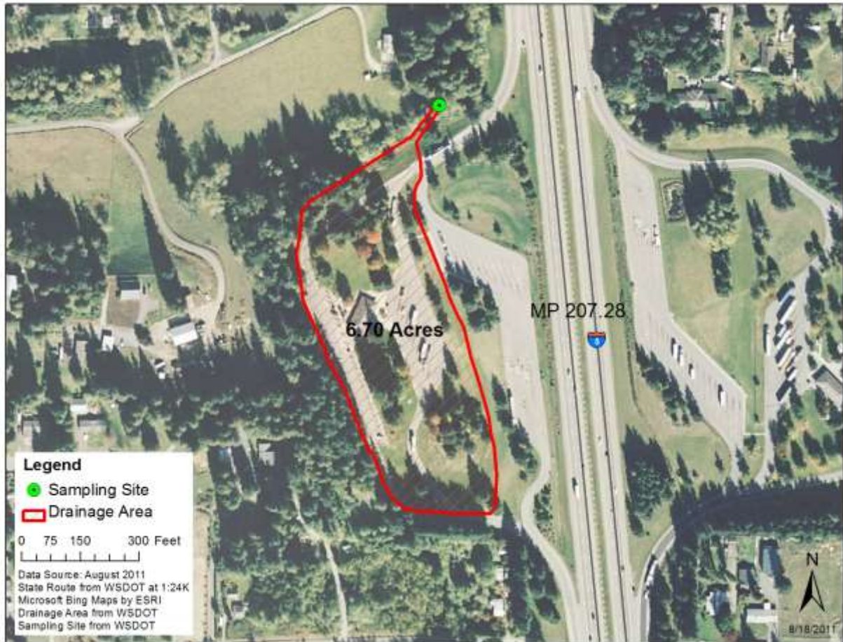
Figure D-8 Smokey Point (SB) Rest Area sampling location and contributing drainage area.
