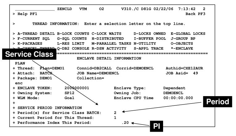
Depending upon how an enclave is created (local allied address space or via DDF) controls what service class, etc that is assigned to a given thread
