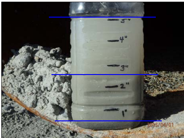
Photo 13. Discharge sample after settling for 5 minutes. The blue lines are used to show sand, silt, and water interfaces.
