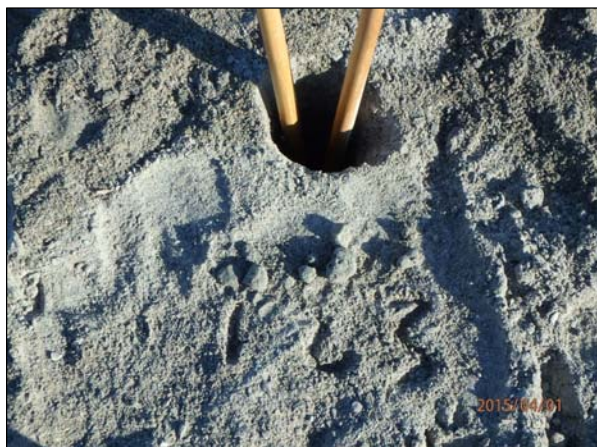
Photo 11. The quantity of rocks within the hole at the center of the constructed berm at Sta. 676+00 between 0-1 feet below existing grade was 3, between 1-2 feet was 4 and between 2-3 feet was 2.
