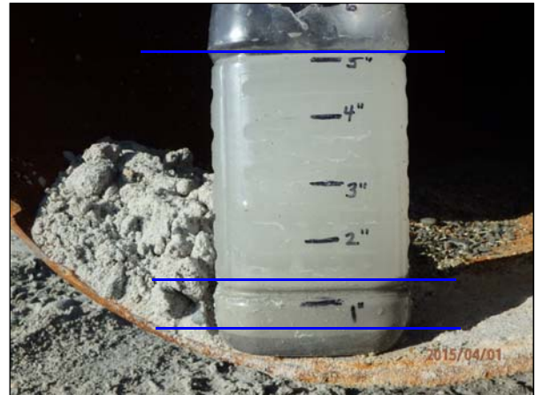
Photo 14. Discharge sample after settling for 15 minutes. The blue lines are used to show sand, silt, and water interfaces.
