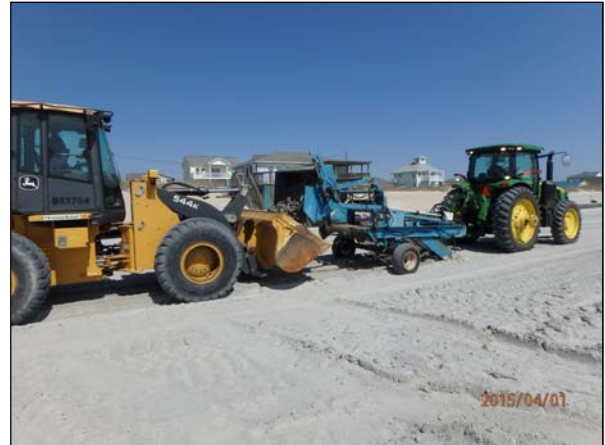
Photo 16. Tigerhole Landscaping emptying the rock picker hopper into a front end loader for removal.
