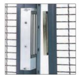
**Electronic Locks** – Electronic locking is an available option. Electronic lock mechanisms actuate on a 12-Volt or 24-Volt signal from the Building Access System (BAS). Electro-Magnetic Lock is used on sliding gates or an Electronic Strike is used on hinged gates.
