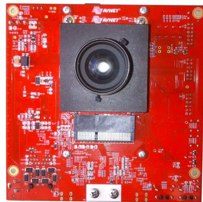
Figure 10: The PYTHON-1300 Camera Module Plugged In the Carrier Card
