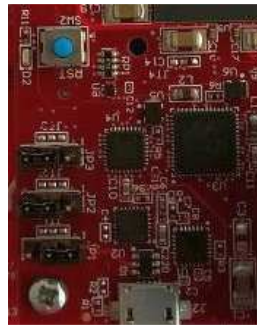
Figure 8: The MicroZed Board Jumpers Settings
