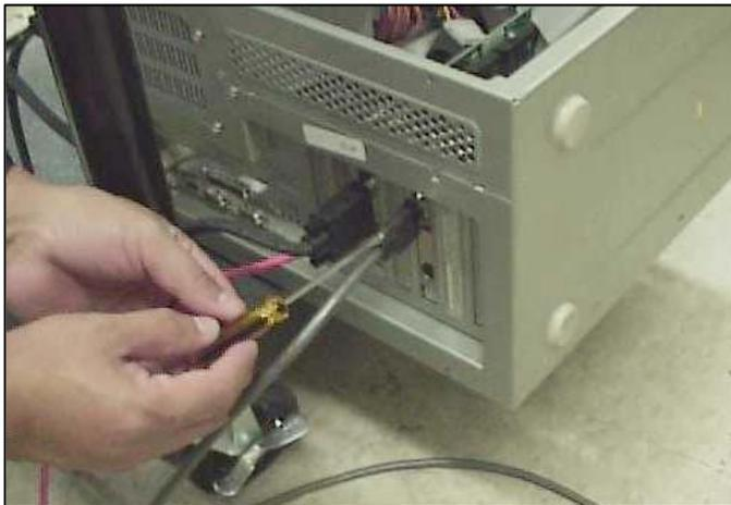
E. Connect the other end of the data cable to the remote module. Then, use a small screwdriver to tighten the screws on the connector.
