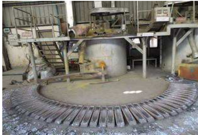
Figure 3.2: Lead Alloying Furnace A and Unloaded Lead Alloy [2].
