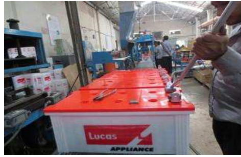
Figure 7.9: Pole Burning with Terminal Post [2].
