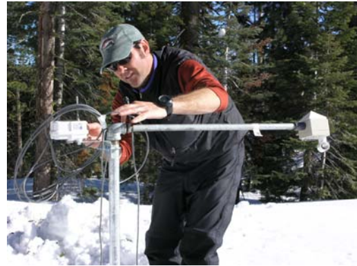
Figure 3. One pod in sensor web that was installed in January 2005 to measure snow depth over a 20,000 m 2 study area at Gin Flat, Yosemite National Park. Depth sensor is on right and wireless pod on left.
