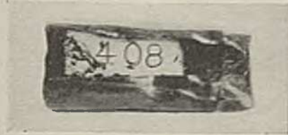
Exploded Detonator Split to Show Numbered Strip
