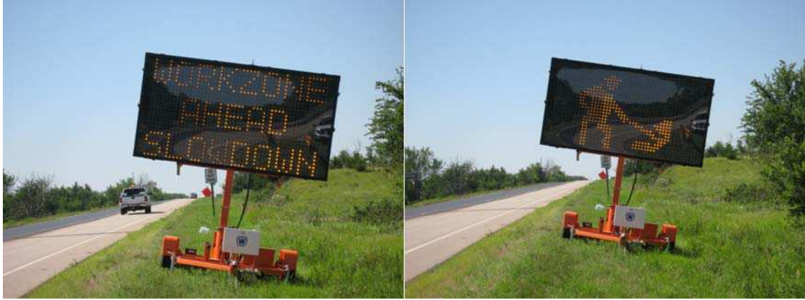
Figure 4.3 Graphic-aided PCMS with the Work Zone Graphic
