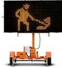
Work Zone Sign on PCMS
