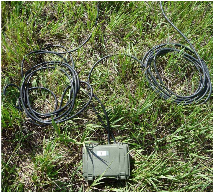
Figure 4.8 A Speed Sensor Connected with Road Tubes
