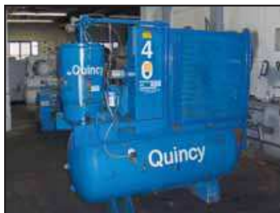
U10828 Quincy QST40 hp rotary screw compressor; tank mounted, 460/3/60; air cooled; excellent condition $6,225.00
