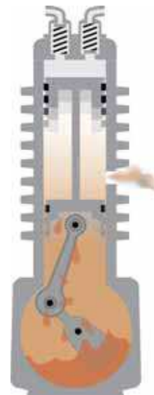
“Oil-less” air compressors control the oil and prevent it from reaching the air end. An important element is the venting of the space between crankcase and air end seals.
