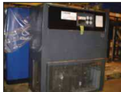
U10246 Zeks 1600 cfm refrigerated air dryer, air cooled, noncycling, 460/3/60; 1999 unit; uses R-22 $8,500.00
