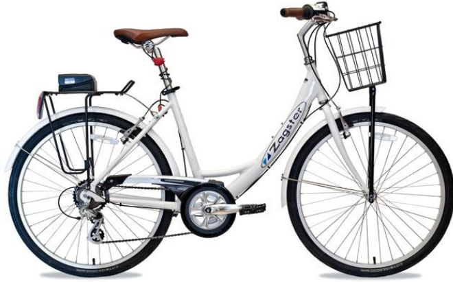
Figure 2 - Typical smart bike with tracking system mounted on rear. Source: Zagster Bike Share
