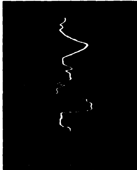
Figure 22. Open-Circuit Voltage From Z_1:Z_2:Z_3 = 1:2:6 , Parallel-Plate Line Mechanically Switched. (a) 2 ns/ small div; 100 mv/div. (b) 5 ns/small div. (c) 10 ns/large div.
