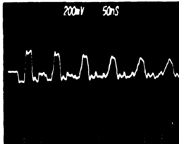
Figure 24. Open-Circuit Voltage From Three-Line Folded Coaxial-Cavity for Small Gap-Spacings.
