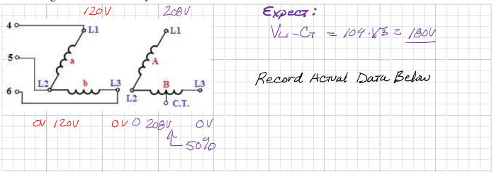
2) Estimate the maximum power this configuration could provide to a 3-phase load, recall that an Open-Delta connected transformers must be devalued.
