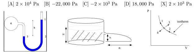
[I.2] A large container has water of density  $\rho$  up to a level H. A small hole is punched on the side at a height h as shown in the figure at the center above. Find the speed v of the water as it emerges from the side hole. Neglect the speed at the top of the tank.
