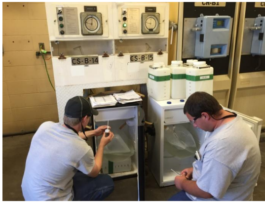
Figure 1. Cory Evers and Matt Pamperin checking to make sure that the refrigerators at the Green Bay Facility are staying at the correct temperature to store the composite sample currently being collected.
