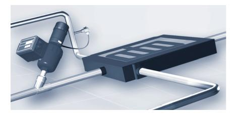
A 2702 control valve with a 1067 local PID controller. The valve is controlling the exit temperature of a media flowing-through a heat exchanger. The process input is a simple temperature transmitter.
