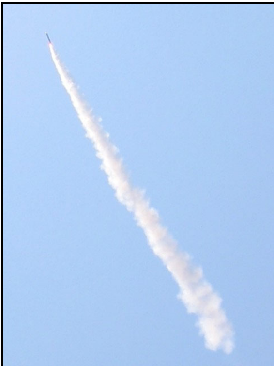
Left: the two H268's can be seen starting up in midair. Right: Andrew e-mailed me this chart recorded by one of the altimeters showing the thrust spikes during flight. A second after burnout of the J400, the two H268's unevenly kicked in. None of the H97's lit. Only one of the G64's lit at the end. (Burney)
