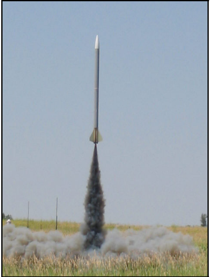
Left: Andrew (left) and George Wimmer prep their Controlled Insanity . Right: Liftoff on a Pro38 J400 Smoky Sam. The rocket was to airstart three, twin sets of motors every few seconds. (Burney)
