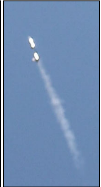
Mobile Rocket Gundam was flown once again on Sunday with a K1100. Unfortunately, drag separation resulted in an early, and messy, parachute deployment. (Left and Right – Burney, Center – Vennard)
