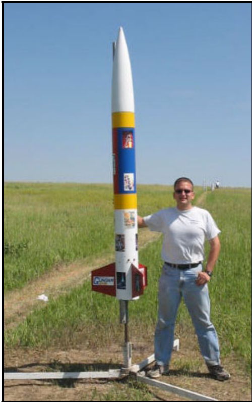
Mobile Rocket Gundam was flown once again on Sunday with a K1100. Unfortunately, drag separation resulted in an early, and messy, parachute deployment. (Left and Right – Burney, Center – Vennard)
