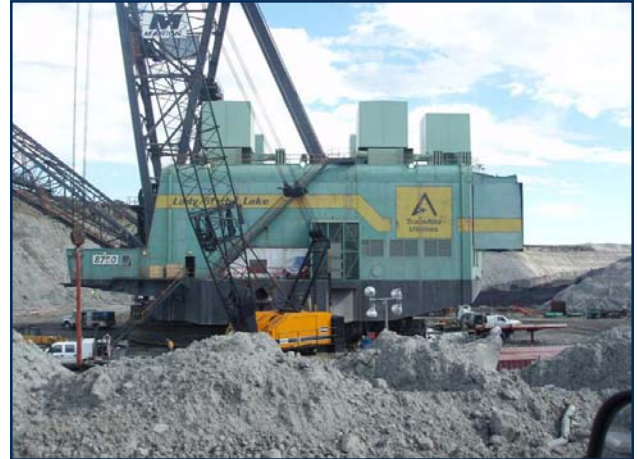
Installation of sound suppression equipment is already complete on TransAlta's 8750 dragline. The large boxes pictured on top of the dragline are fan shrouds and they help suppress the noise of the dragline.
