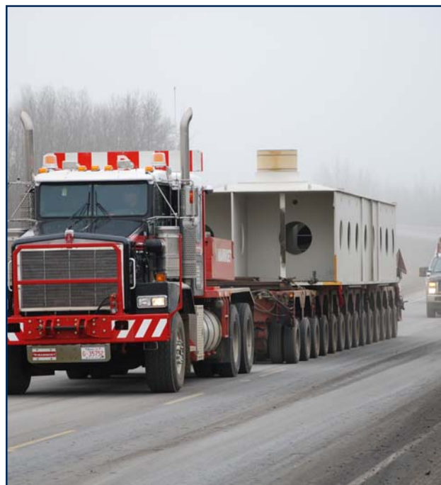
In April the largest centre section of the 7,200 tonne dragline arrived on site via truck from Acheson where it was shipped from its manufacturer in Wisconsin by rail to begin the assembly process.
