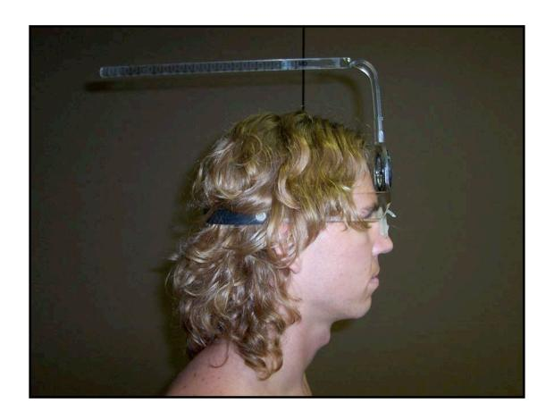
Figure 3. Measuring rounded shoulders with a T-bar
