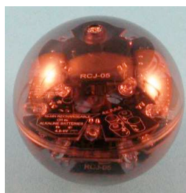
Figure 6.3:HiTechnic IR Ball
