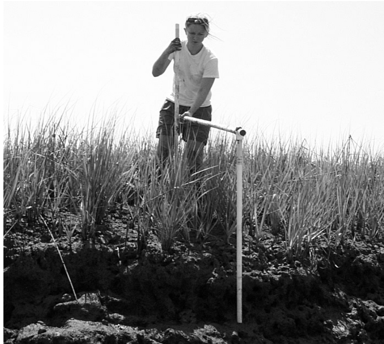
Figure 7: Field measurements of shoreline change. A measuring stick was used to reset the seaward pole and landward pole to a distance of 1 m apart.
