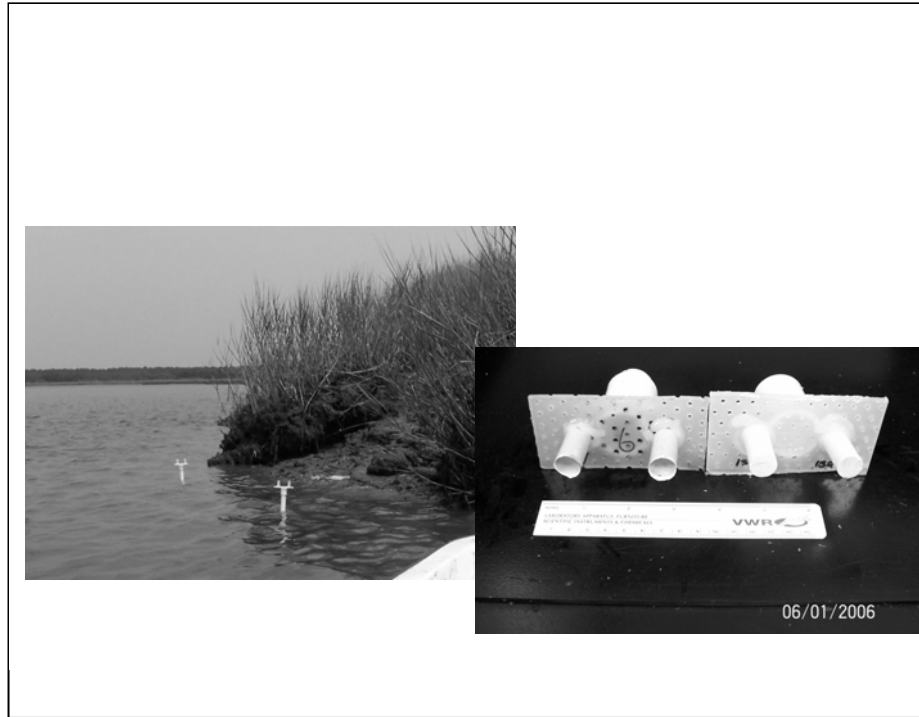
Figure 19. Long-term flow was measured through plaster dissolution techniques. Plaster cylinders were deployed at low tide (left photo) and retrieved after three days. Plaster cylinders were weighed pre and post deployment. (Right photo) Post deployment cylinders are on the left and pre deployment cylinders are on the right. Plaster dissolution is used as a surrogate for flow.
