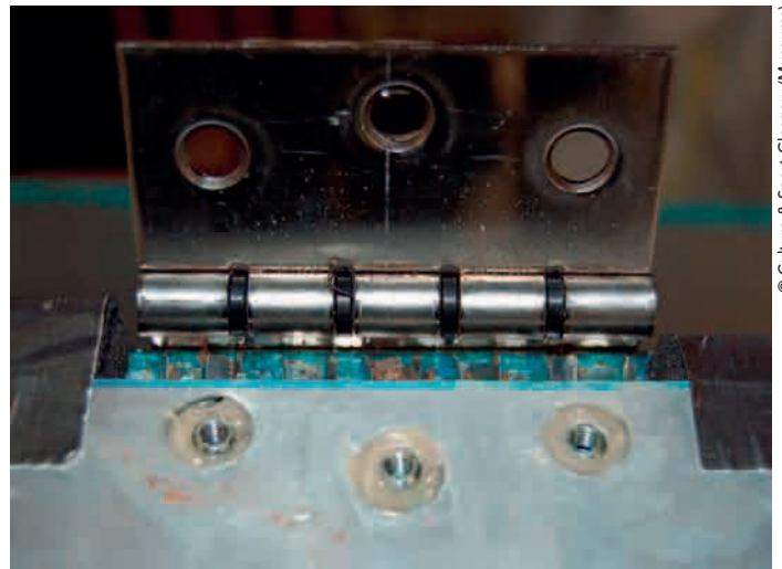
Detail of the fixing for the Hexlite box, showing the hinge open, with the threaded inserts secured in the epoxy resin
