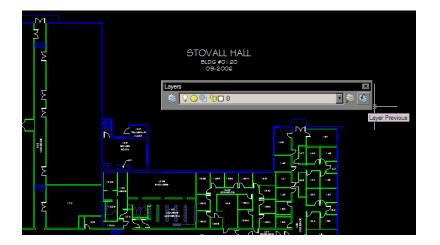
STEP FIVE: Once you have successfully converted all old layers to the new Master layer scheme, you will need to purge all old layers and blocks to clean the drawing. Type "purge" in the command line to initiate the Purge dialog box.
