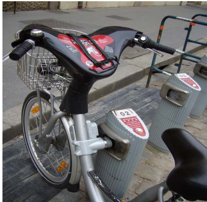
Bike sharing system locking mechanism
