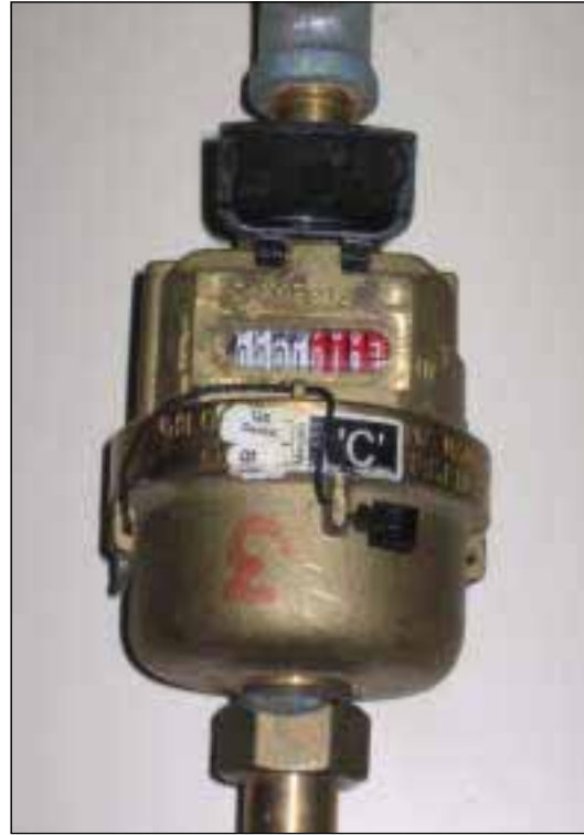
Figure D2: Photos of test apparatus used in South Africa. Class “C” meters were used for the check meters.
