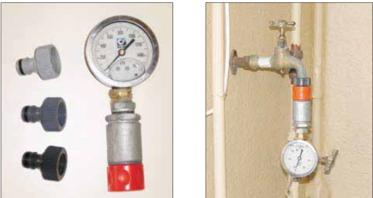
Figure F-1: Photos of a typical pressure test apparatus
