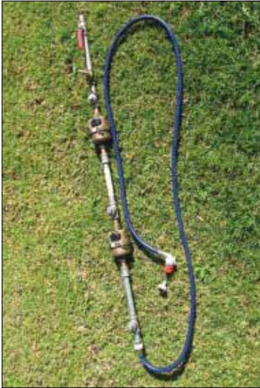
Figure D2: Photos of test apparatus used in South Africa. Class “C” meters were used for the check meters.
