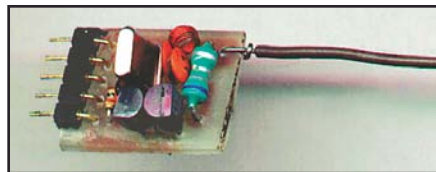
Figure 4—Transmitter module ready to plug into a control and sensor module.
