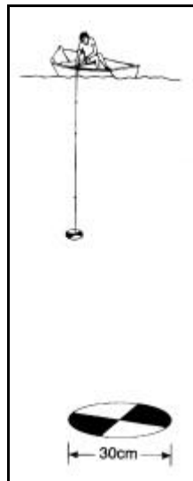
Figure 5. The use of a secchi disc to assesses vertical water clarity. The secchi disc is lowered into the water until the black and white quarters are no longer distinguishable. The length of rope from the surveyor to the disc is then recorded. Source: English et al. (1997).
