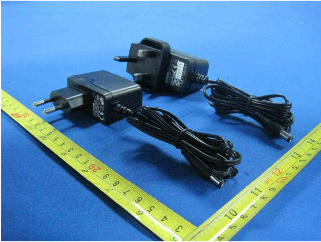
Fig.7 - Over view of approved external Power Supply
