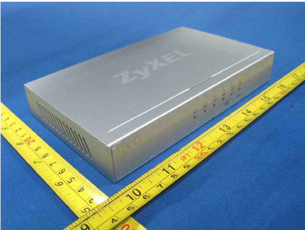
Fig.2 - Front and side view of model GS-105B v2 (Overall: approx. 163mm x 100mm x 26mm)
