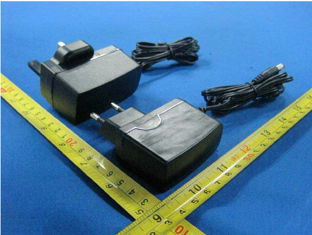
Fig.8 - Over view of approved external Power Supply
